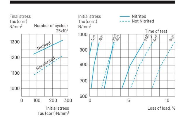
In diagram 1 the fatigue properties of this grade are illustrated in a Goodman-diagram, based on a special test spring design.
