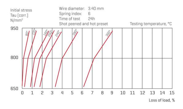
Diagram 2-3 show the relaxation properties (loss of load) of springs made from GARBA 177 Supreme® subjected to three different stress levels at different temperatures.
