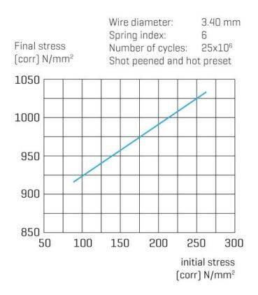
In diagram 1 the fatigue properties of GARBA 177 Supreme® is illustrated in a Goodmandiagram, based on a special test spring design.
